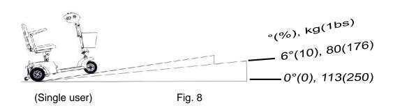
Angles and weights shown here for this scooter indicate the safe working angles for the user and equipment. Any scooter used outside these parameters may be unsafe and or cause future problems with the electrical systems
