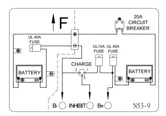
Battery Wiring Diagram (for 22Ah)
