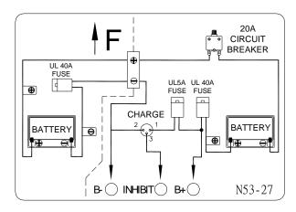
Battery Wiring Diagram (for 14Ah)
